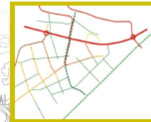
The road network / a fine network ensuring a high level of access and a road system that slows down the traffic flow.
